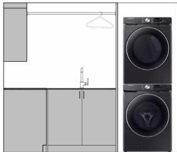
Planned Laundry Room Elevation
